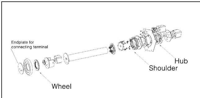
Figure 5. Robot's (version 2) Leg assembly
