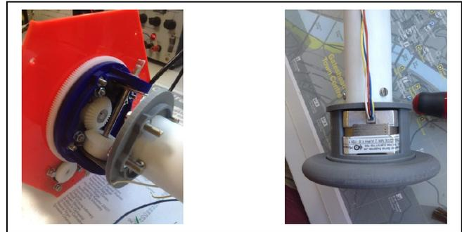
Figure 6. Prototype 2 details of the Hub & Shoulder joints (l), and wheel joint (r).
